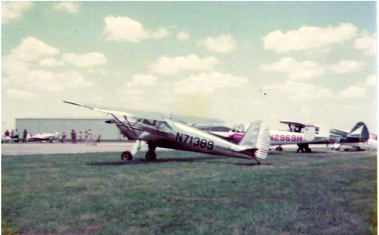
Luscombe 8A, fabric wing, single fuel tank in fuselage, 65 HP
