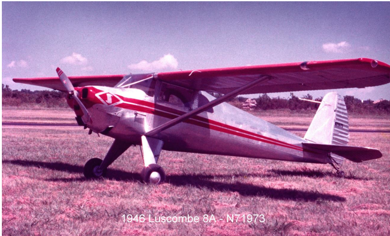
Model 8A, serial number 3400, metal wing, 2 wing fuel tanks, 75 HP
